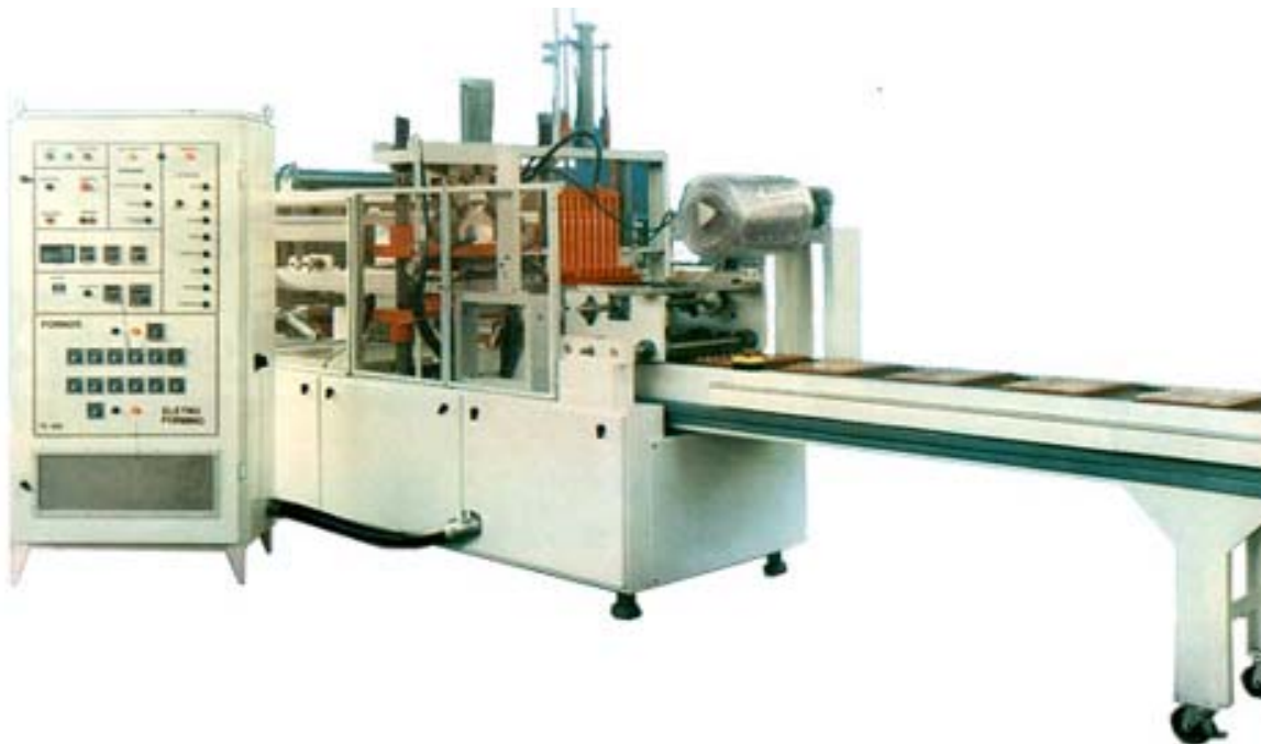
TC + BLISTERPACK – Molding and bubble cutting station
